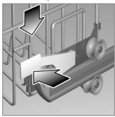
To lower the basket, press in succession the two levers on the left and right sides of the basket. Always take hold of the side of the basket on the upper edge, otherwise the basket will not drop smoothly (and may damage the utensils).
